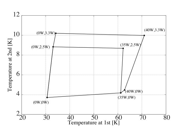
Fig3: Measured typical load map of the Cryocooler Unit.
