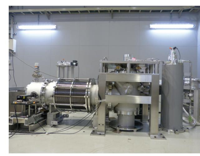
Pic1: Cryocooler Unit
