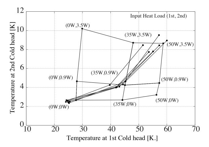
Fig1: Measured load map of the PT cryocoolers.
