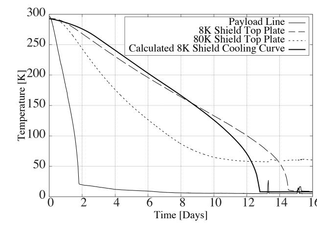
Fig6: Typical cooling time of the cryostat with estimated cooling curve.
